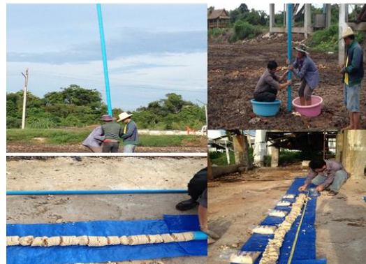
Photo 2. Taking samples of the contents of the pit
